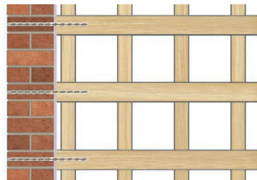
Restraining gable walls using mini retrofit purlins and BowTies
