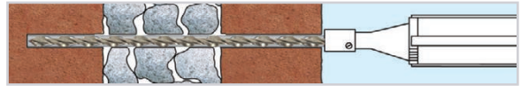
2. Push CemTie fully into grout-filled pinning nozzle of grout gun and insert nozzle to the back of the hole
