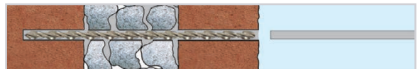
4. Back pressure pushes nozzle out of hole to leave fully grouted tie
