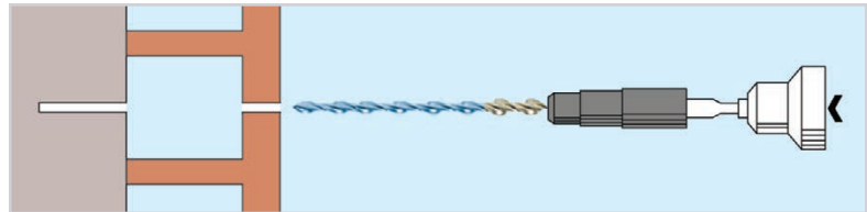
2. Load the tie into the insertion tool fitted to an electric hammer drill (SDS type)
